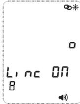
If “Linc OFF” is displayed, press the test button (check mark), to turn it on. To turn the Link Light off, press the test button until Linc OFF
