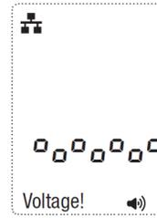
Data Cable, High Voltage detected! Disconnect immediately to prevent damage to the tester
